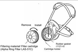
\*DO NOT disassemble the used filter cartridge. Dispose of it in a sealed bag, etc. so that hazardous substances do not diffuse. Clearly indicate that the bag contains "waste plastic" or "waste glass and ceramics." Inform the industrial waste disposal operator that hazardous substances are attached to the used filtering material and ask for a proper disposal.
