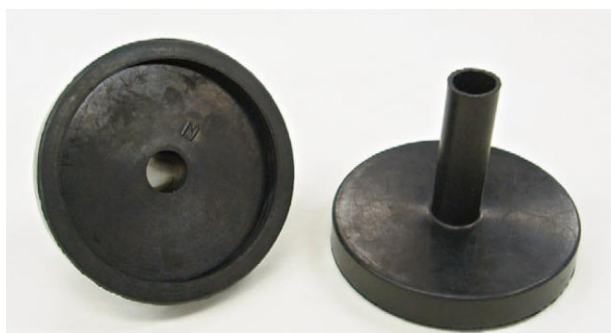
*Fit checker (made of rubber) to close off the air inlet hole
